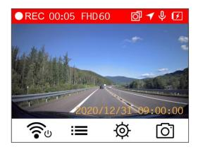
After the car engine is switched off, the DrivePro will automatically save the current recording and power it off.
