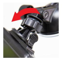
**5.** After the DrivePro is in the best position, turn the adjustment knob clockwise to make sure that the DrivePro is securely locked in place.
